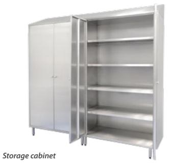
Welded stainless steel frame structure with braced doors. With 4 fixed shelves, inclined top. Wall-mounted with adjustable front legs. Closes with a ball and spring stop. Options: Safety lock with 2 keys, stainless steel closing plate.
